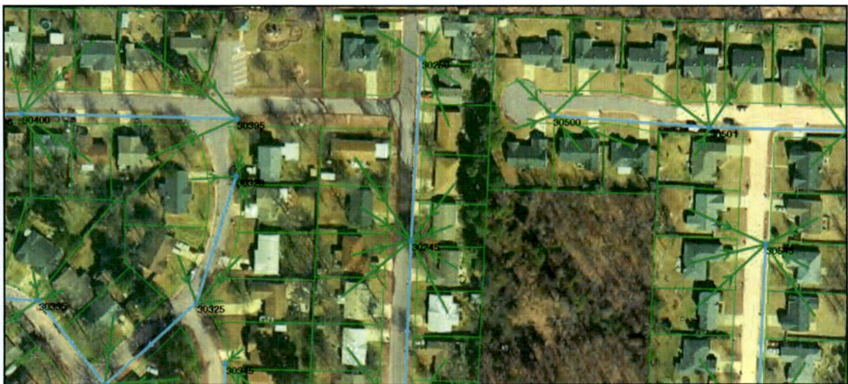
Figure 2.5 – Sub-catchment Drainage Links
