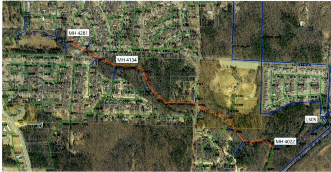
Figure 3.10- Gravity Line from MH 4281 to MH 4022
