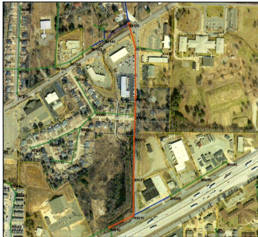
Figure 3.8- Gravity Line from MH 30125 to MH 30010
